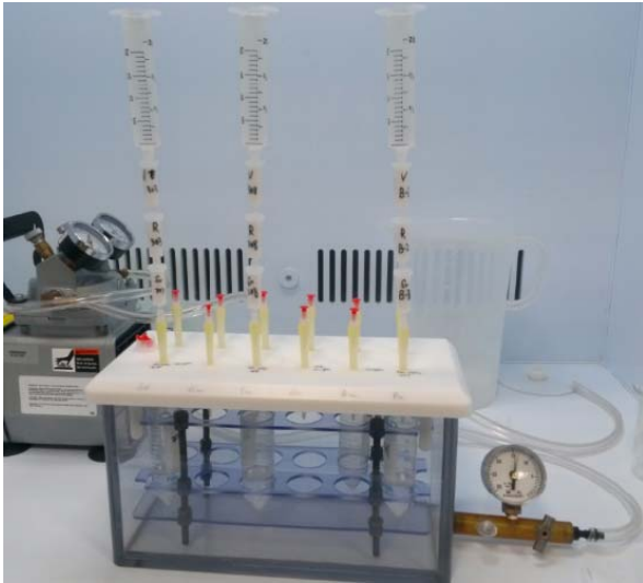
Fig. 2. Ion exchange chromatography resin to extract target radionuclides emitting alpha and beta particles.
