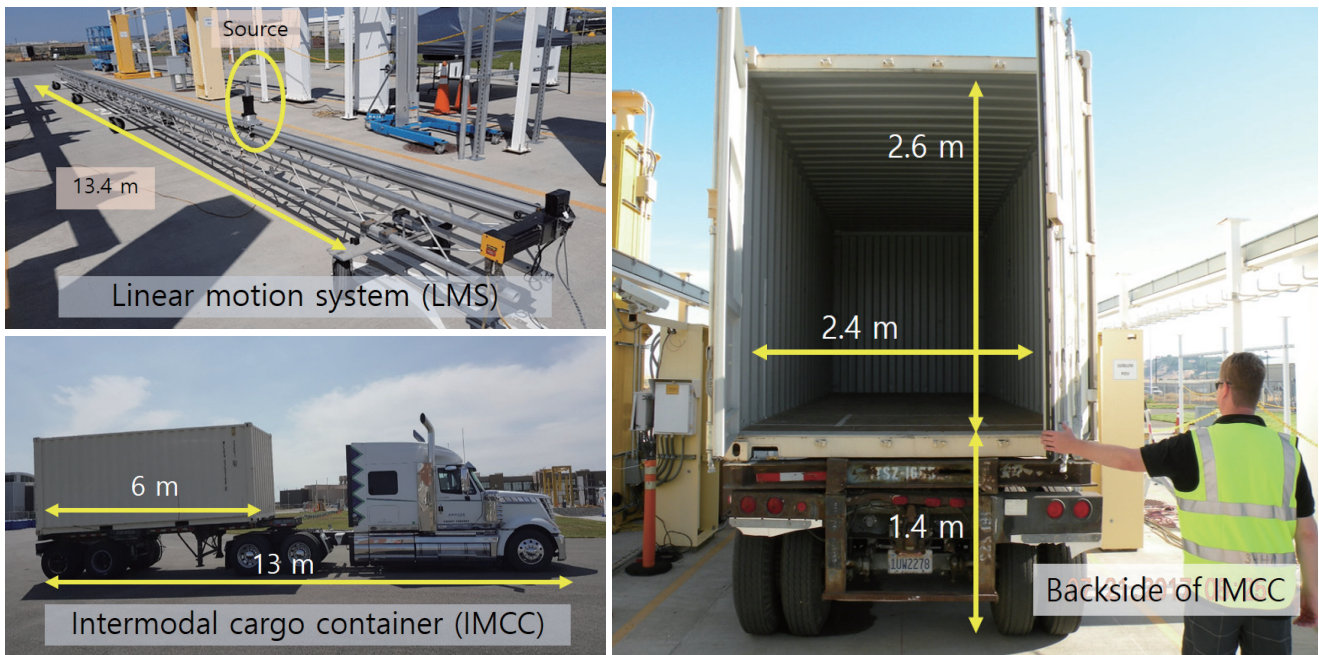
Fig. 7. Sources for spectrum measurement were set in motion by LMS and IMCC.
